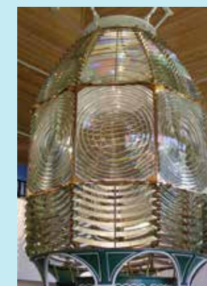
Fresnel Lens Assembly placed on a turntable that rotates around a lamp or light source.
